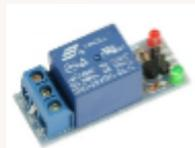
Figura 3. Modulo relay <https://www.colombianizate.com.co/tienda/arduino/arduino-rele-relay/modulo-rele-1-canal-5v-arduino/>
